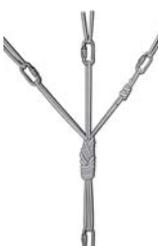
An anchor in its simplest form may have steel bolts at the top which you can clip into with screw-gate carabiners. A length of quality 11mm static rope then traverses the distance between the bolts and the edge of the cliff. The static rope is tied-off and two (preferably steel) carabiners are placed in an opposite and opposed manner which the climbing rope is then threaded through and the climber ties on to.
